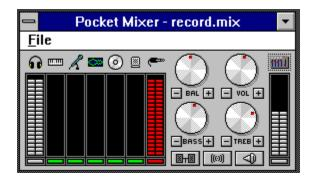
This arrangment will allow you to record from the LINE IN input on the card. This can be your CD, tuner, record player or whatever is plugged in there. To record using a microphone, plug it in to the MIC IN jack and click on the MIC ICON located on the bottom right of the PocketMixer and bring up the slider under the small MIC ICON (3rd from left). Click on the small green bar located at the bottom of that slider and it will turn red. That means RECORD MODE.
